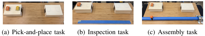
Fig. 2. Task setup. 2(a): The pick-and-place task is to move both objects onto the other shelf. 2(b): The inspection task is to first move the object along the blue line and then place it on the other shelf. 2(c): The assembly task is to first move the object to the other shelf, then grasp the orange block on the pipe and slide the pipe through the lamp.
